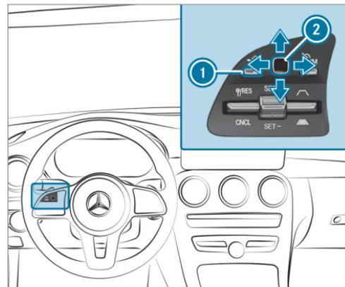
The on-board computer is operated using left-hand Touch Control **2** and the left-hand back/home button **1**.
